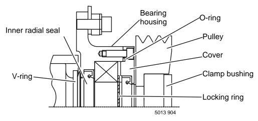
Check that the shaft journal and bearing housing are undamaged.
